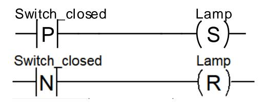
Reads : if the switch is closed activate the lamp for one cycle Implicit action : if the switch is open do not activate the lamp
